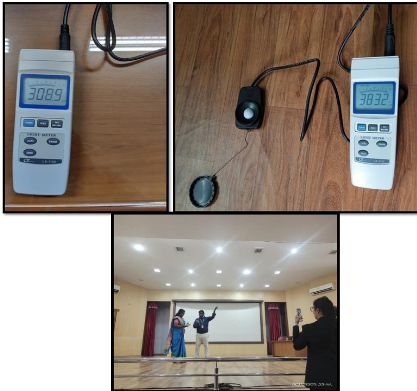
Light Intensity Measured at various locations of Adichunchanagiri Institute of Technology, Karnataka
